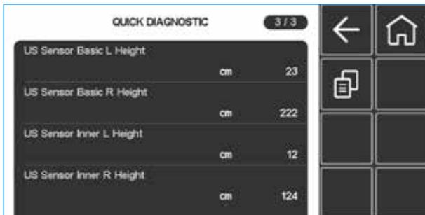
This section displays an overview of all boom position data and measurements:
