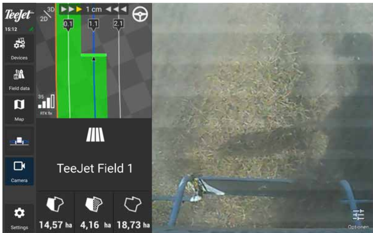
Figure 19: Camera view in the main window (right) and guidance lines in the Mini View (left)
