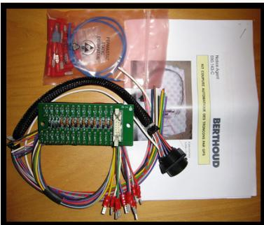
If the DP Tronic controller has no BoomPilot interface installed from the factory or the BoomPilot interface installed, is of an older type than described above, it's necessary to install Berthoud no. 292 483 or TeeJet no. 902-422, before using Teejet kit no. 990-888 or 990-889.
