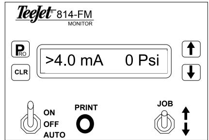
If a pressure transducer is NOT being used, press the R key to skip this step and advance to the next programming step.
