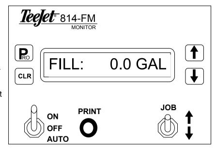
During the filling process you can temporarily close the filling valve by turning the master switch back to the OFF position. The filling is continued after switching back to the AUTO position. When the desired volume is reached the console will automatically close the filling valve (disengage the pump).
