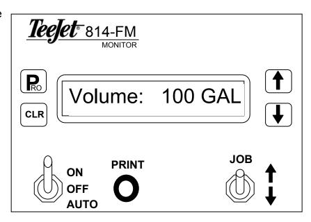
Note: To achieve an accurate flow meter calibration, a volume of at least 50 gallons should be pumped during calibration. The more volume used for calibration the more accurate the flow meter will be.
