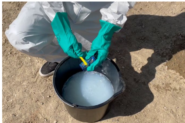
Cleaning of the strainers with a TeeJet brush
