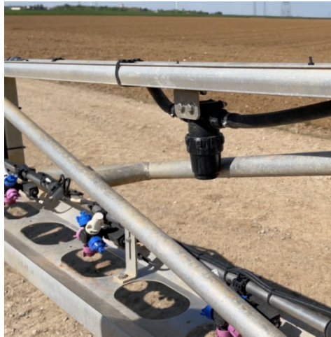
Spray boom strainer cleaning
