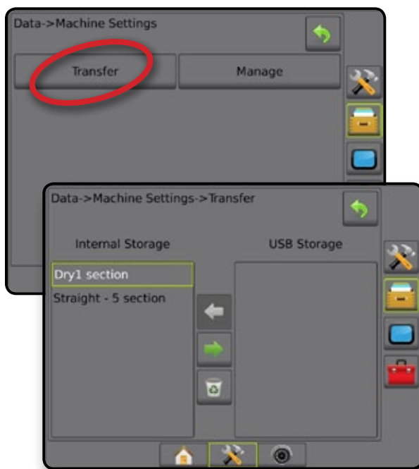
Figure 1-38: Machine Settings – Transfer
