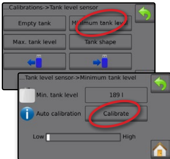
Figure 35: Tank level sensor – Minimum tank level
