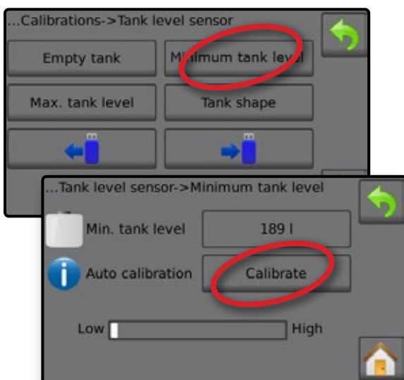
Figure 3-28: Tank level sensor – Minimum tank level
