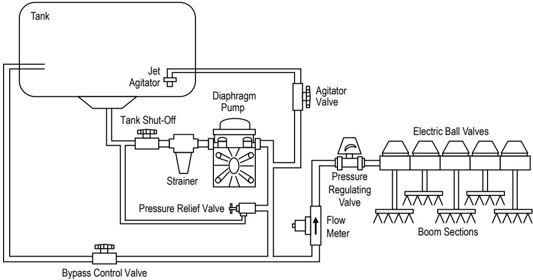
Figure 1-6: Throttle Plumbing Diagram, Pressure Based System, Diaphragm Pump
