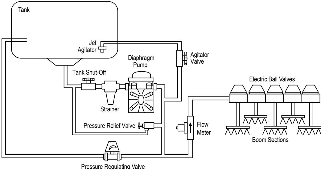
Figure 1-4: Bypass Plumbing Diagram, Pressure Based System, Diaphragm Pump
