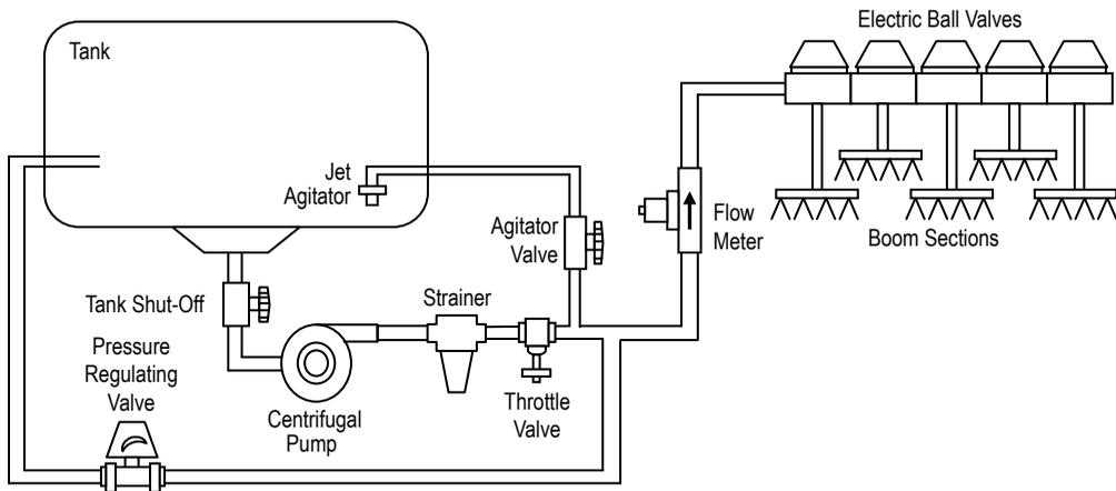
Figure 1-2: Bypass Plumbing Diagram, Pressure Based System, Centrifugal Pump
