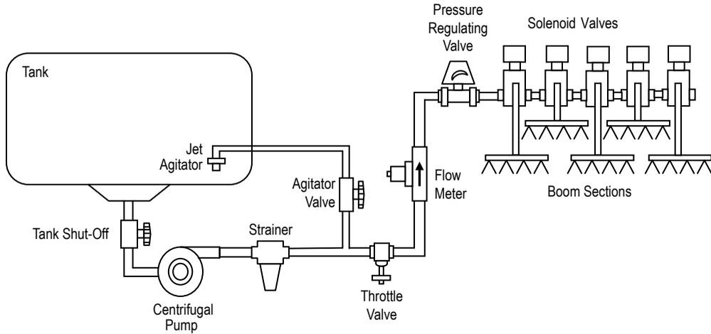
Figure 1-8: Throttling Plumbing Diagram, Pressure Based System, Centrifugal Pump
