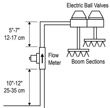
Figure 1-11: Flow Meter Examples
