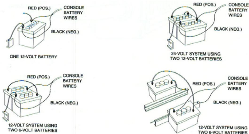
Reliable operation of the 844 Sprayer Control depends on a clean power supply. Ensure this by connecting the power cables directly to the battery and not to another power source.
