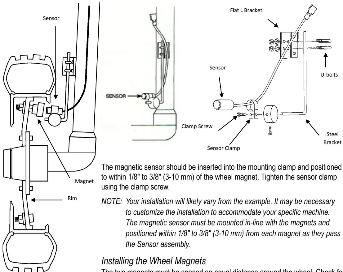
The magnetic sensor should be inserted into the mounting clamp and positioned to within 1/8" to 3/8" (3-10 mm) of the wheel magnet. Tighten the sensor clamp using the clamp screw.
