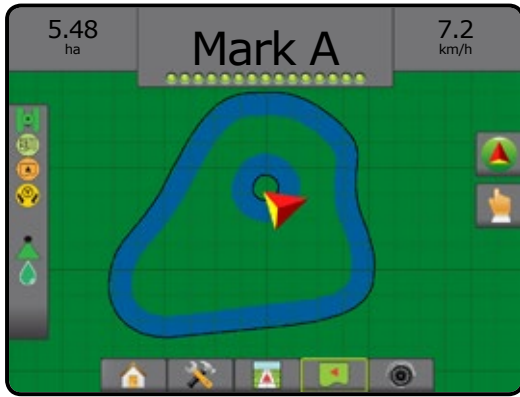
Figure 7-25: Add Interior Boundary
