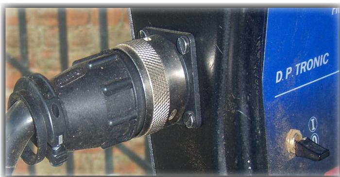
Make a hole in the left part of the plastic housing and install the round connector. The Hole should be  $\varnothing 25$  mm and fixing holes  $\varnothing 3.2$  mm.
