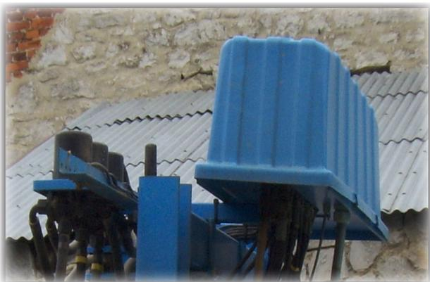
Fix the relay box to the frame
