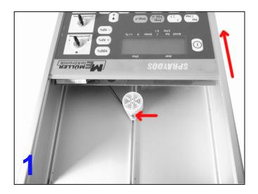
Unscrew the top and bottom endplate of the SPRAYDOS controller.
