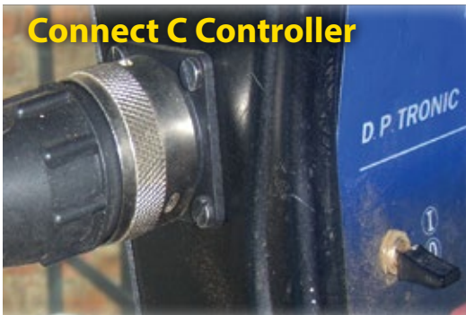
Figure 8: BoomPilot harness to flow control harness
