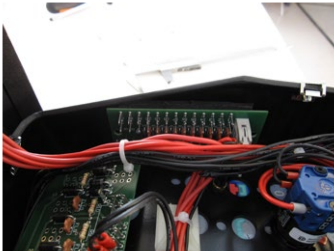
Figure 6: Installing the Connector
