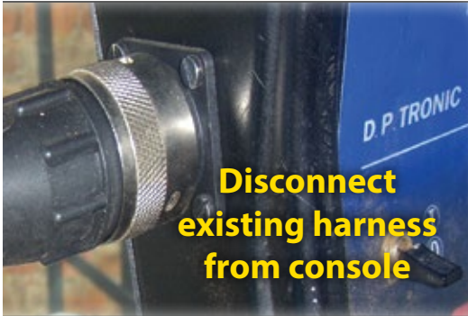
Figure 8: BoomPilot harness to flow control harness
