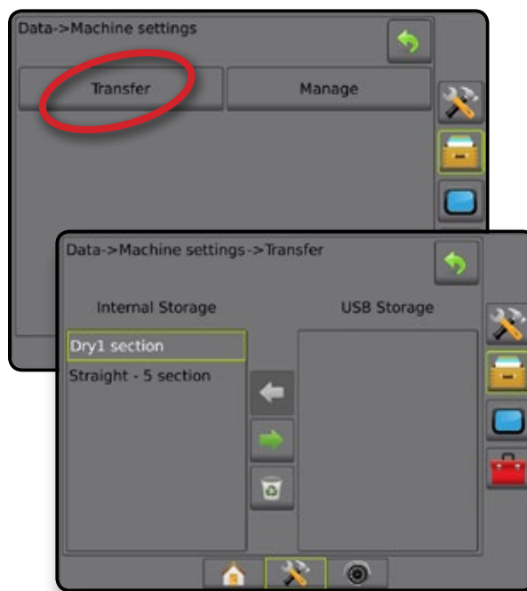
Figure 4-38: Machine settings – transfer
