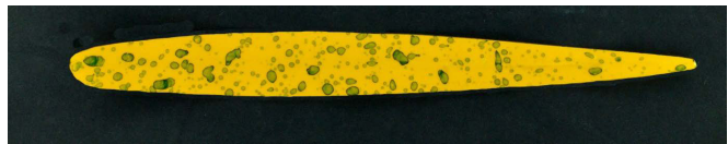
Deposit on artificial cereal leaf: TeeJet AITTJ60
