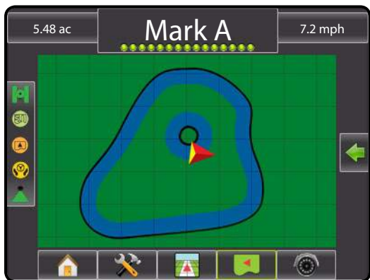
Figure 7-56: Add Interior Boundary
