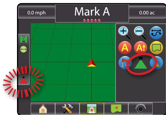
Figure 7-62: Automatic to All Sections On Mode
