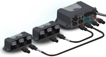
Spray Job Computer for advanced spray control and feature unlocks
