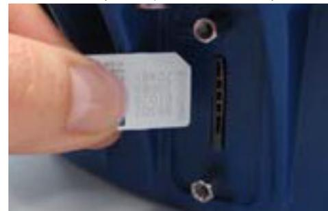
The SIM connector is a push-in/push-out type. If the SIM is correctly installed, its outside edge will be essentially flush with the surrounding enclosure metal surface.
