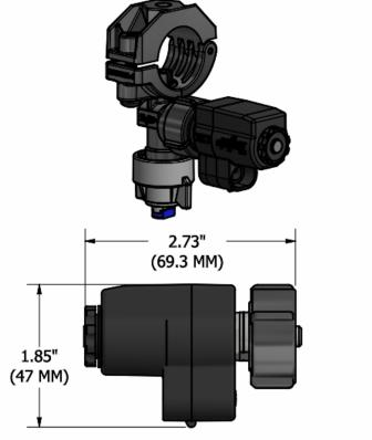
NOTE: IT IS RECOMMENDED TO INCLUDE A LINE STRAINER OF 80 MESH OR FINER WITH ALL 6-CHEMSAVER® APPLICATIONS
