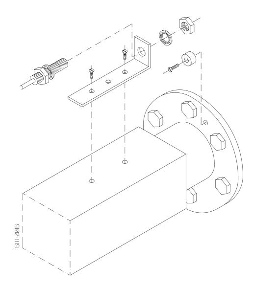
The wheel sensor can be fitted to the cardinal shaft on 4-wheel drive machines.
