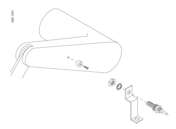
The implement sensor can be fitted in other positions (PTO handle, hydraulic cylinders, other handles, etc.). There must be movement of minimum 50 mm. The distance between the sensor and the magnet must not exceed 5 mm.
