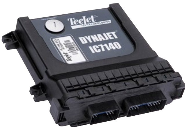
Figure 1-1: DynaJet IC7140 Controller
