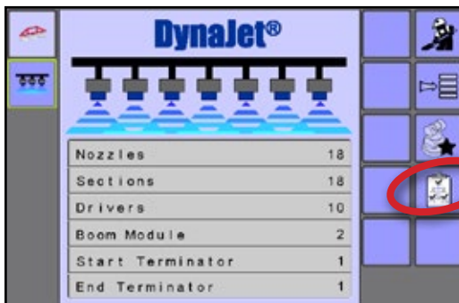
Figure 8-3: System Overview – Through the Home Screen
