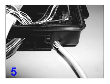
Place the free wires of the ARAG 180 adapter cable one by one in the hole and pull the cable trough as shown.
