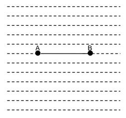
The solid line represents the reference line created with points A & B. The dashed line shows that parallel lines are automatically created on the left- and righthand side plus in front of and behind the reference line. This means that parallel guidance **is** possible outside the points A and B
