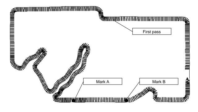
The first pass is almost finished and the marks for the reference line have been created (mark A & B) for which the rest of the field will be driven parallel to. See steps 7, 8, & 9 in the above for marking the reference line).
