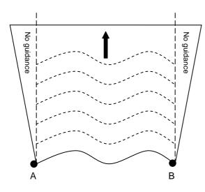
The solid line represents the initial reference line created with points A & B. The dashed lines show that parallel lines are automatically created in front of the initial reference line.
