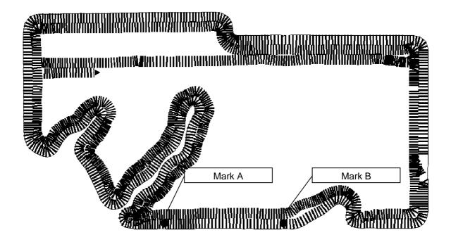
The second pass around the headland is finished and work has started parallel to the straight reference line, which was created with marks A & B during the first pass around the headland.
